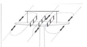
Recommended measure: Switches should be attached below the crossarm, and the wires insulated.
