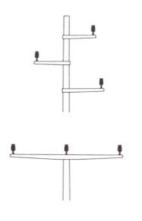
In wet weather **wooden poles** with upright insulators can be a hazard as well as poles that are grounded. For mitigation, the top of armless poles has to be well above the uppermost wire (right).
