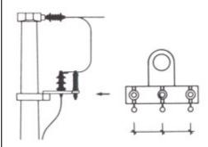
Frequently over voltage reactors extend above the tops of terminal poles and tower stations. This hazard for birds can be avoided if the over voltage reactor is attached below the crossarm and all down leading wires are insulated with tubing.
